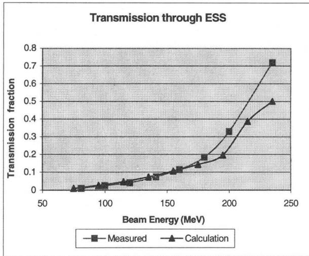
Figure 5 Beam Transmission through the ESS
