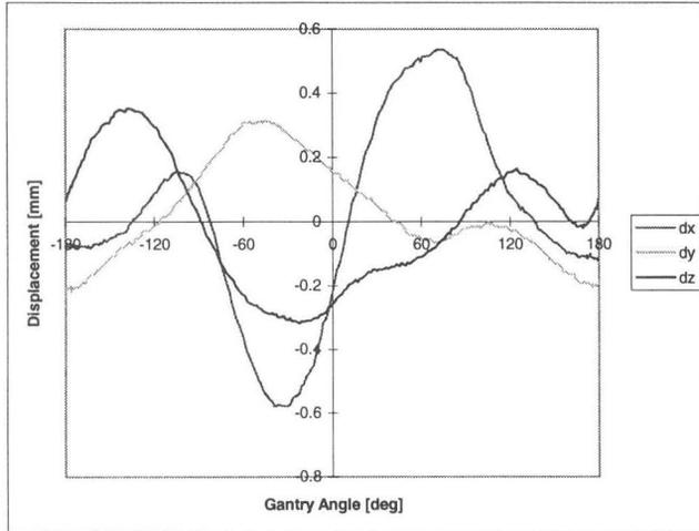
Figure 8 Measurements of Gantry Contribution to Deviation of beam to position compared to isocenter
