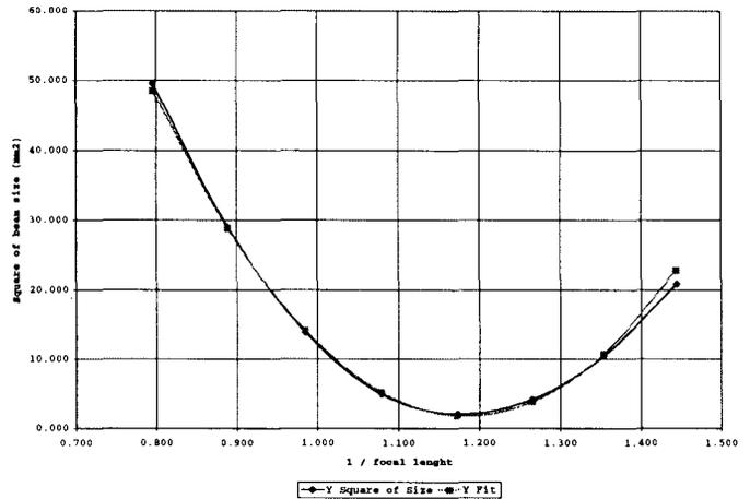
Figure 3 Vary Quad measurement of beam phase space
